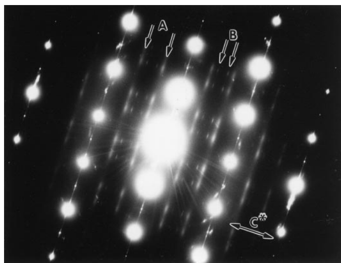
FIG. 2. Electron diffraction pattern of \text{In}_{0.40}\text{Nb}_3\text{Se}_4 showing the (1\bar{1}0)^* reciprocal lattice plane at 90 K. A slightly diffuse set of superlattice spots occurs along rows such as indicated by arrows at A and a second, sharper, set of superlattice spots occurs along rows such as indicated by arrows at B.
